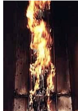
Vertical Cableway Fire Test NSWCCD (Uncoated Cable)
