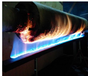
IBP undergoing successful 3 HR Flame Test (Not passed by cables)
